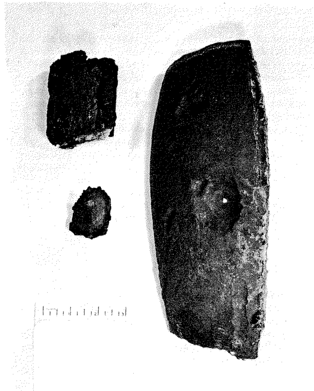
Figure 1. Large piece is perforated Type 316 stainless steel elbow section from naphtha pyrolysis furnace outlet line. Small round chunk is a porous oxide plug which had formed directly over hole. Also shown is a square piece of soot-contaminated asbestos insulation.
