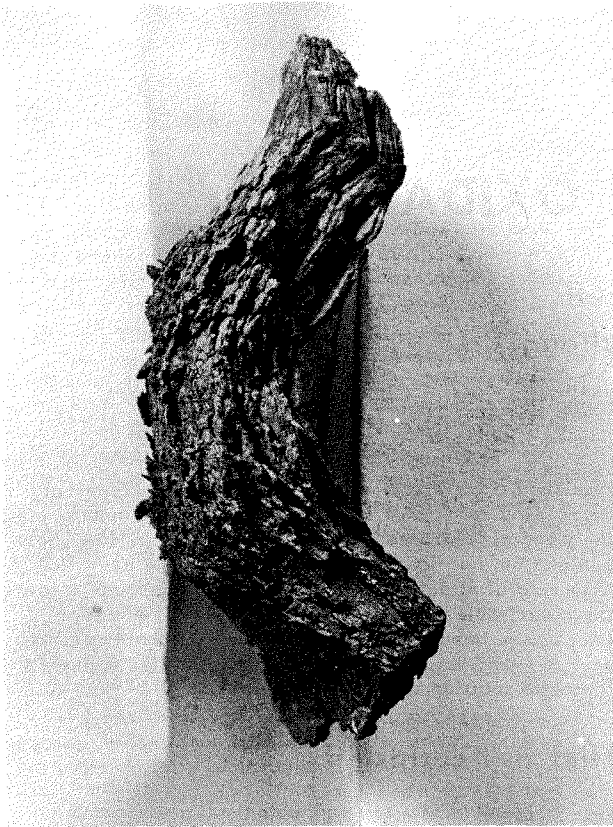
Figure 2. Cross-sectional view of bulky oxide plug shown in Figure 1. Stratified appearance and friable nature of corrosion product is characteristic of catastrophic oxidation.
